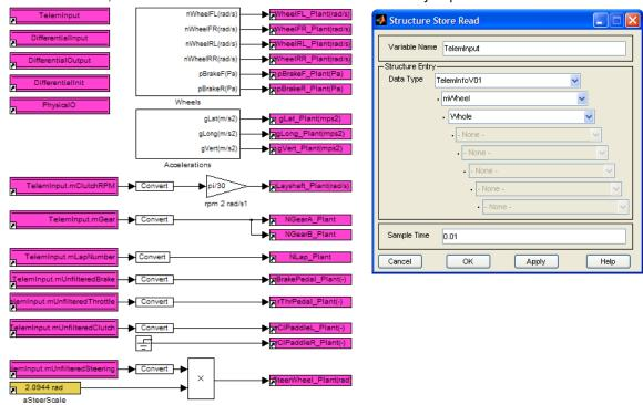
The following example shows how the individual wheel information can be extracted:
