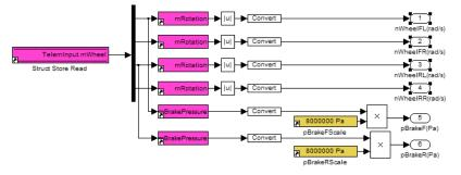
Each of the call-back functions available in rFactor-Pro can be access in Simulink as function called subsystems to tie in with the appropriate calculation step of the rFactor simulation:
